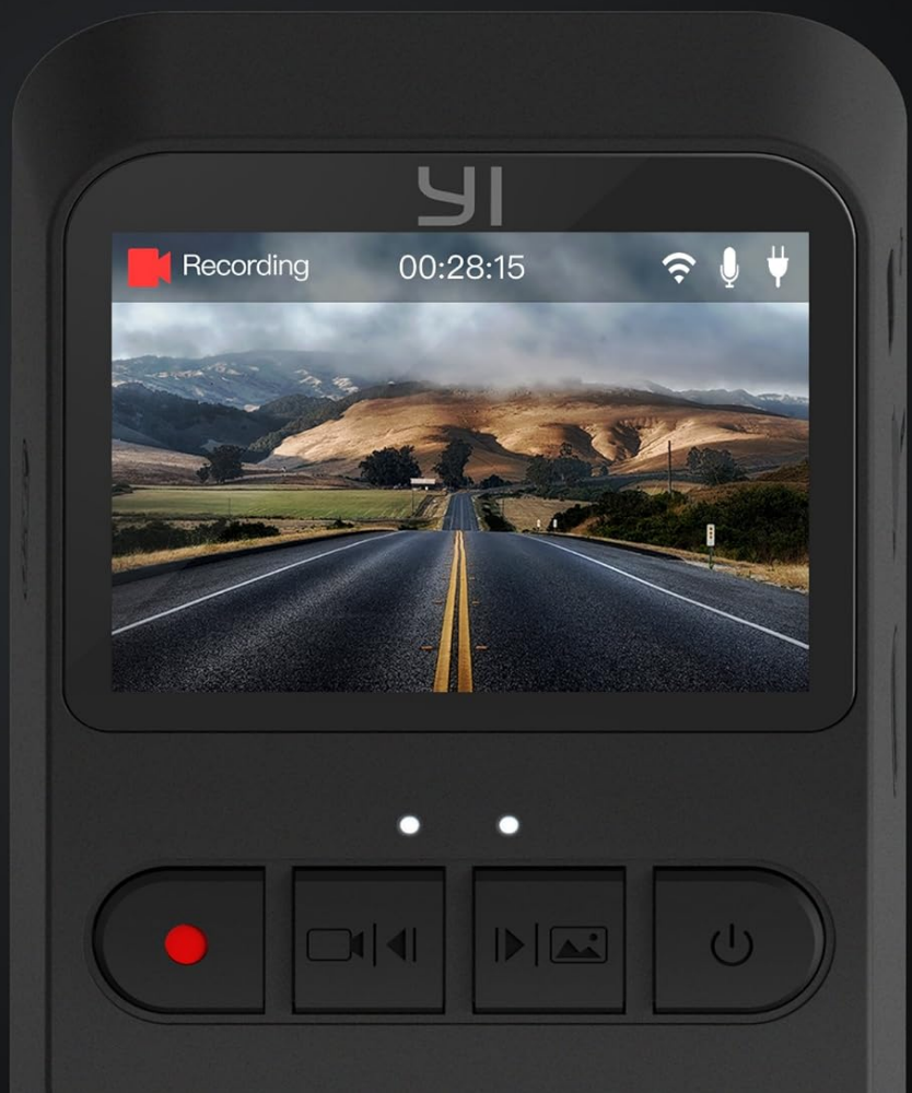
Figure 4.2: The intuitive 2-inch LCD screen of the YI Mini Dash Cam C1B showing a live view of the road.
