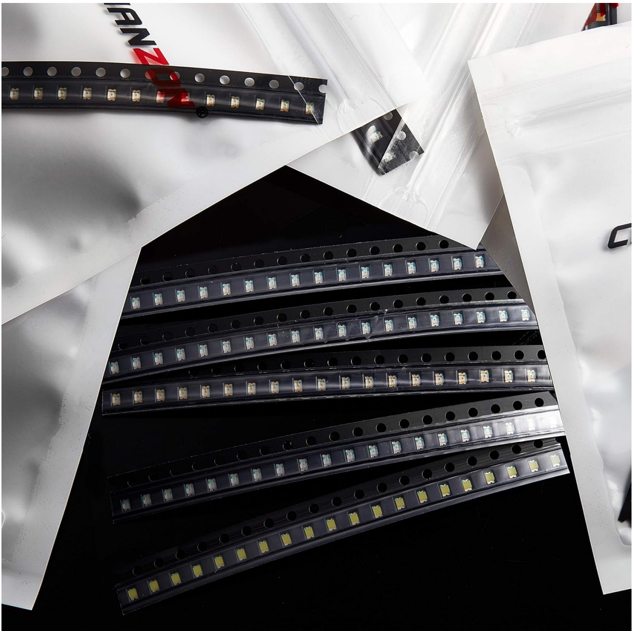
Image 4: This image provides a close-up view of the 0805 SMD LEDs mounted on their tape reels. The LEDs are visible in various colors, demonstrating their compact size and how they are presented for use in automated pick-and-place machines or for manual handling in electronic projects.
