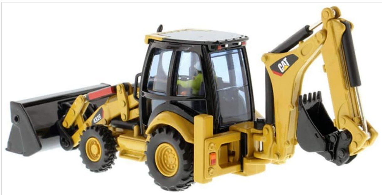
Image 4.3: Side view demonstrating the adjustable stabilizers.
