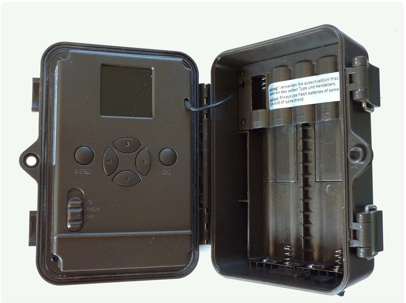
Image: The camera opened, revealing the battery compartments on the right and the display and control buttons on the left, along with the SD card slot.
