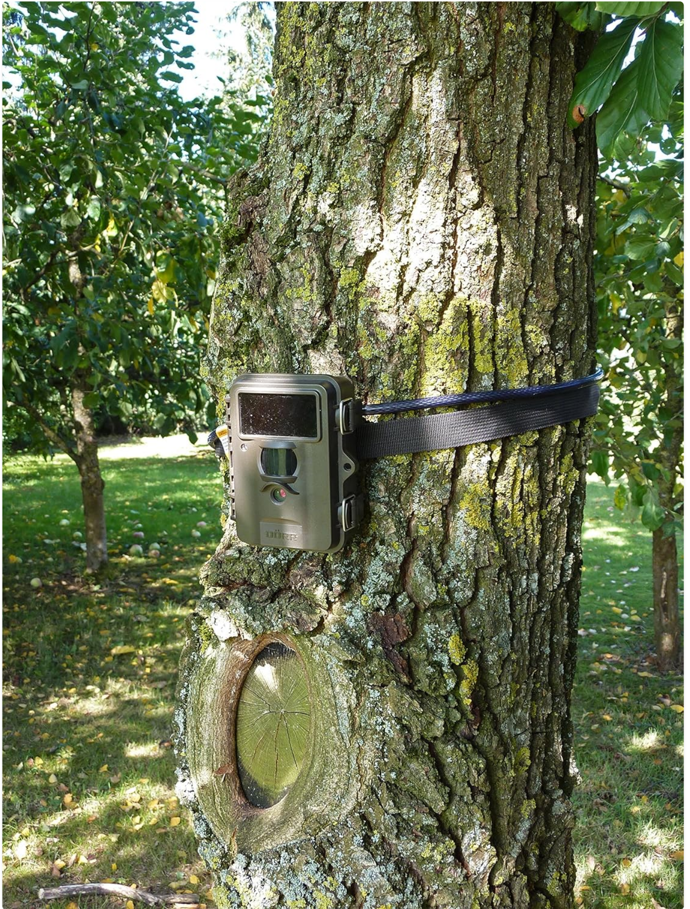
Image: The camera securely mounted to a tree trunk using the black nylon strap.
