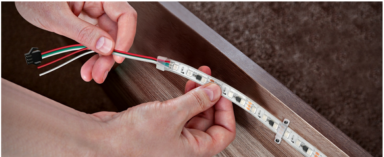
Figure 7: Connecting the power/data wires to the LED strip.
