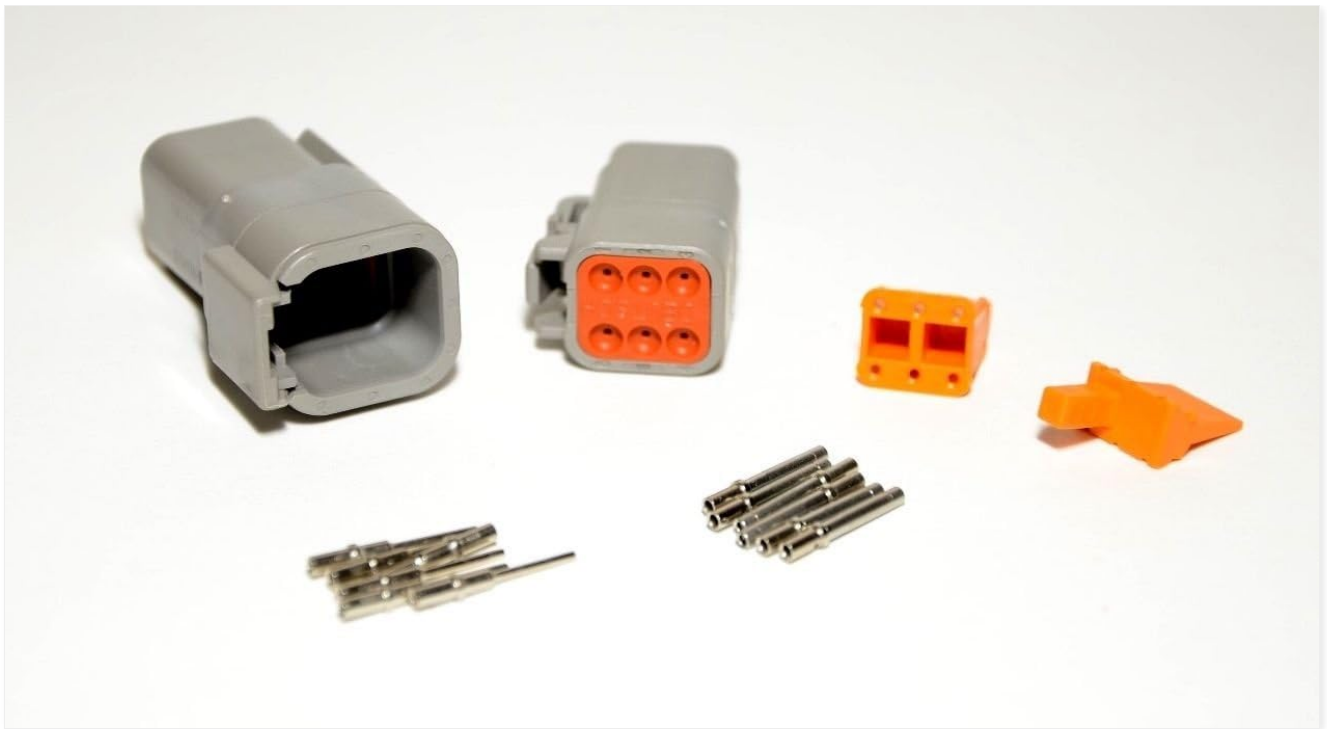
Figure 1: Components of the Deutsch DTM 6-pin connector kit, including male and female housings, orange wedges, and solid contacts for 20AWG wire.
