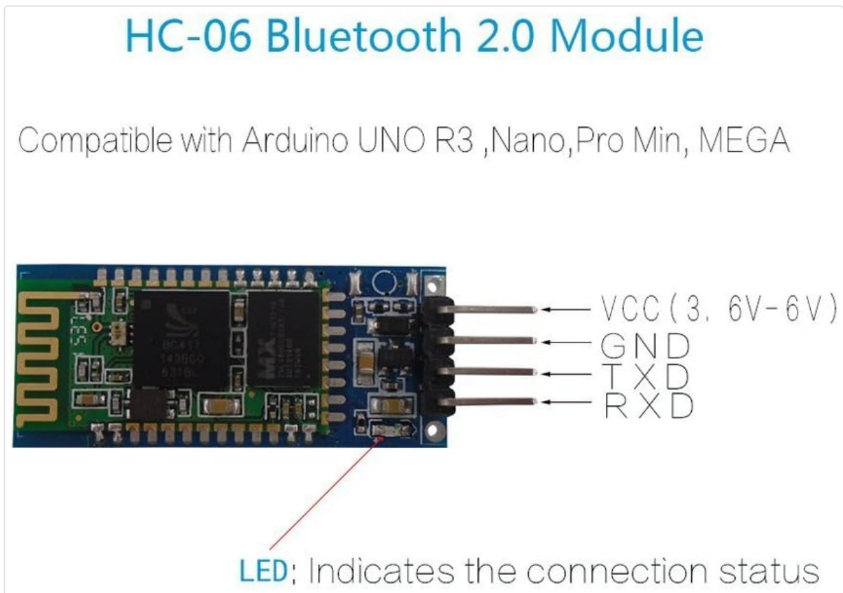
Figure 2: Pinout diagram for the HC-06 Bluetooth module. This diagram clearly labels the VCC, GND, TXD, and RXD pins, along with the LED indicator for connection status.
