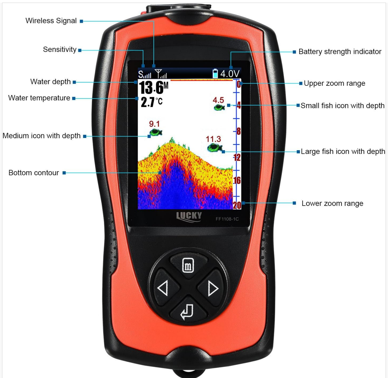
Image: A detailed view of the fish finder's display, with various indicators and readings clearly labeled, including water depth, temperature, fish icons, and bottom contour.
