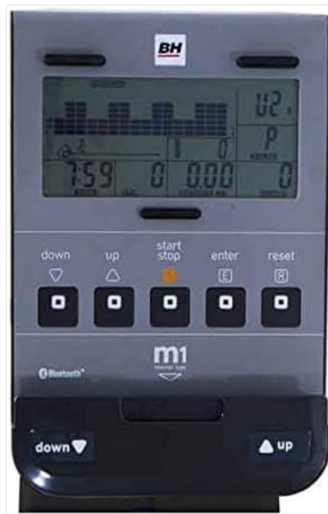
Image 4.2: Another view of the rower's console, highlighting the control buttons. This image shows the 'down', 'up', 'start/stop', 'enter', and 'reset' buttons for navigating the console's features.
