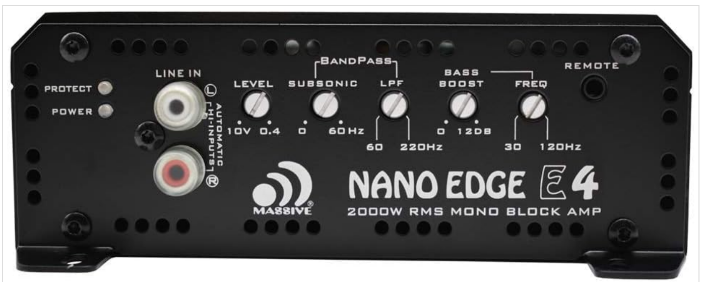
Image 6.1: Control panel of the amplifier, highlighting the input and adjustment knobs for optimal sound configuration.
