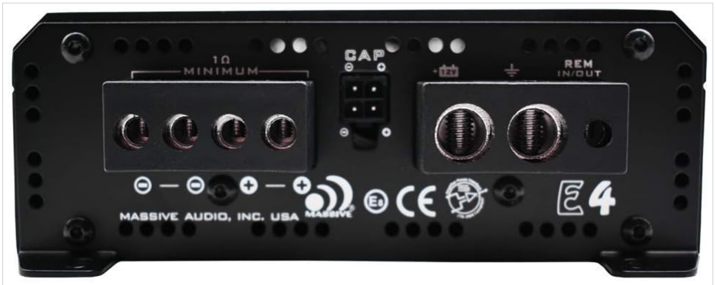
Image 5.2: Rear panel of the amplifier, detailing the power, ground, remote (REM IN/OUT), and speaker output terminals. Note the 1 Ohm minimum impedance marking.
