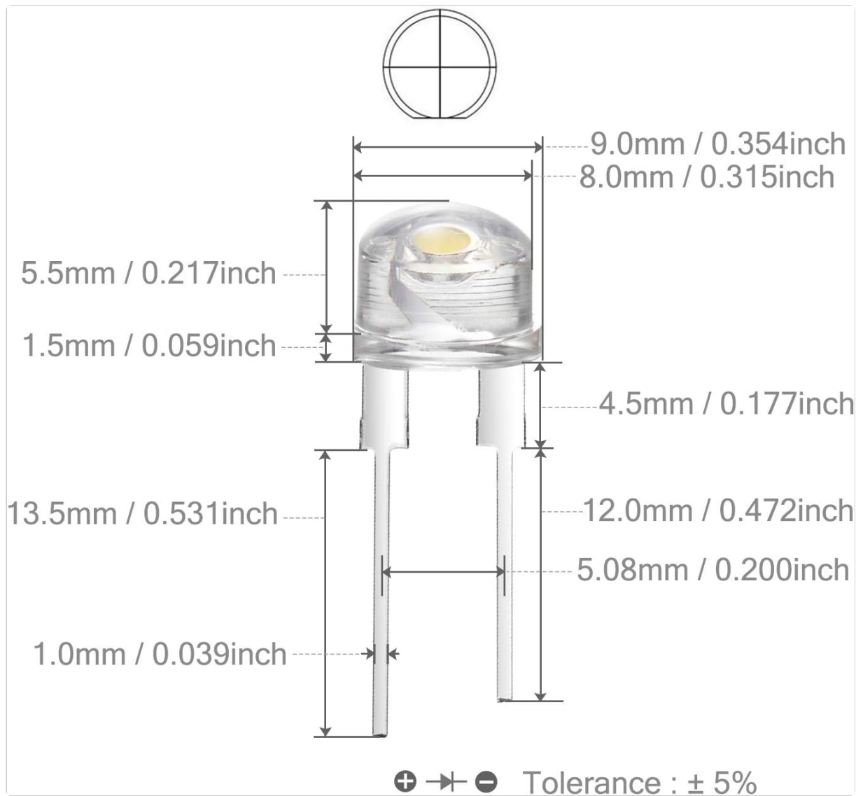
Image: Detailed dimensions of the 8mm straw hat LED diode, including lead length and spacing.
