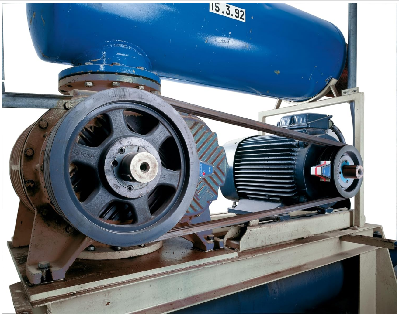
Image: The SKF TKBA 40 laser alignment tool being used on large industrial machinery, demonstrating its applicability in real-world operational environments for precise pulley alignment.
