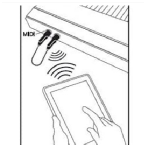
Image: A diagram illustrating the wireless connection of the MD-BT01 adapter from a musical keyboard to a tablet device.
