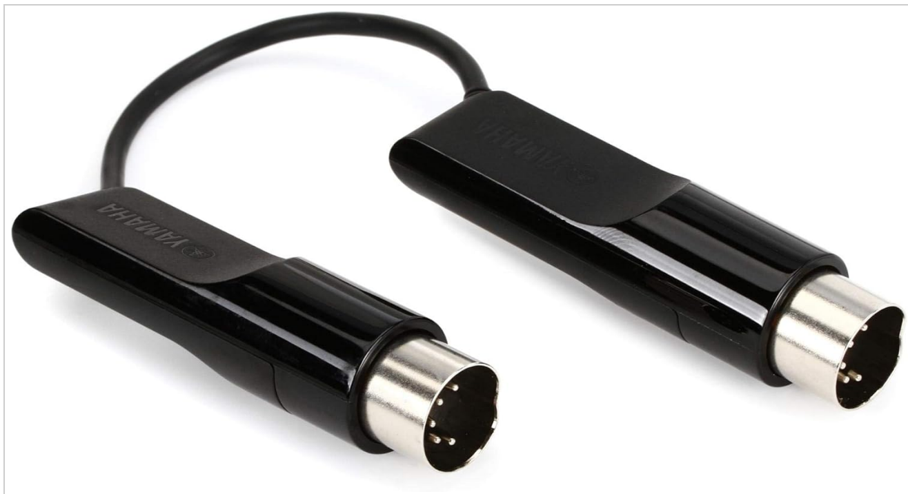
Image: The Yamaha MD-BT01 adapter, showing its two 5-PIN DIN connectors designed for MIDI IN and MIDI OUT ports on a musical instrument.
