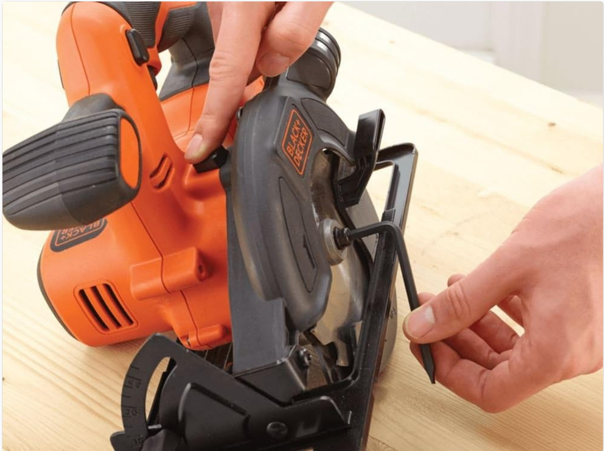
Figure 3: Demonstrating blade installation using the spindle lock.
