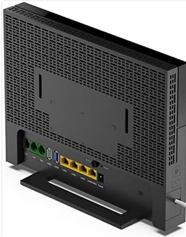
Figure 4.2: Rear view of the ZTE Tim Hub+ modem, displaying the various connectivity ports.
