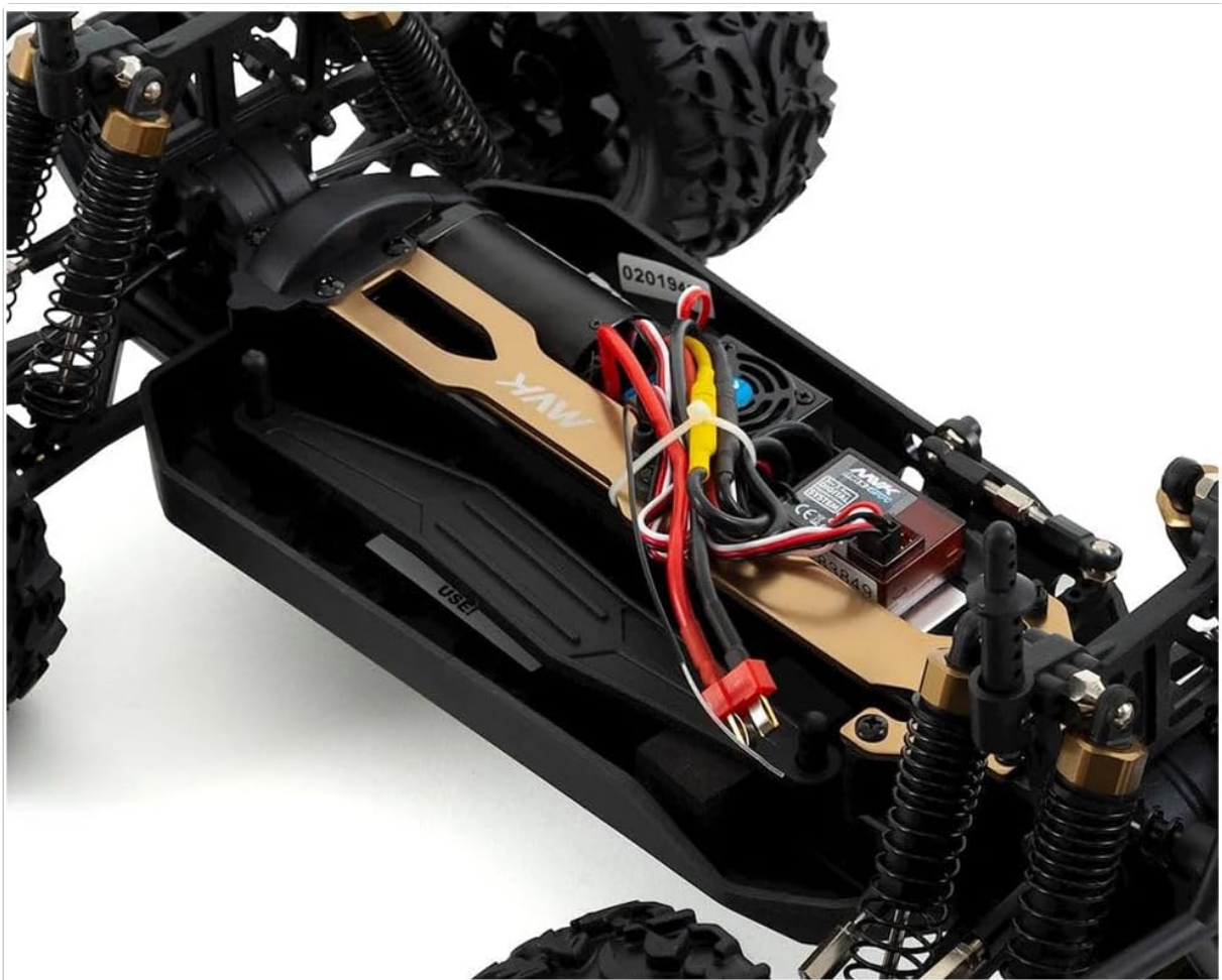
Figure 4: Detailed view of the Maverick Strada MT chassis, showing the layout of the electronic components including the battery tray, electronic speed controller (ESC), and receiver.
