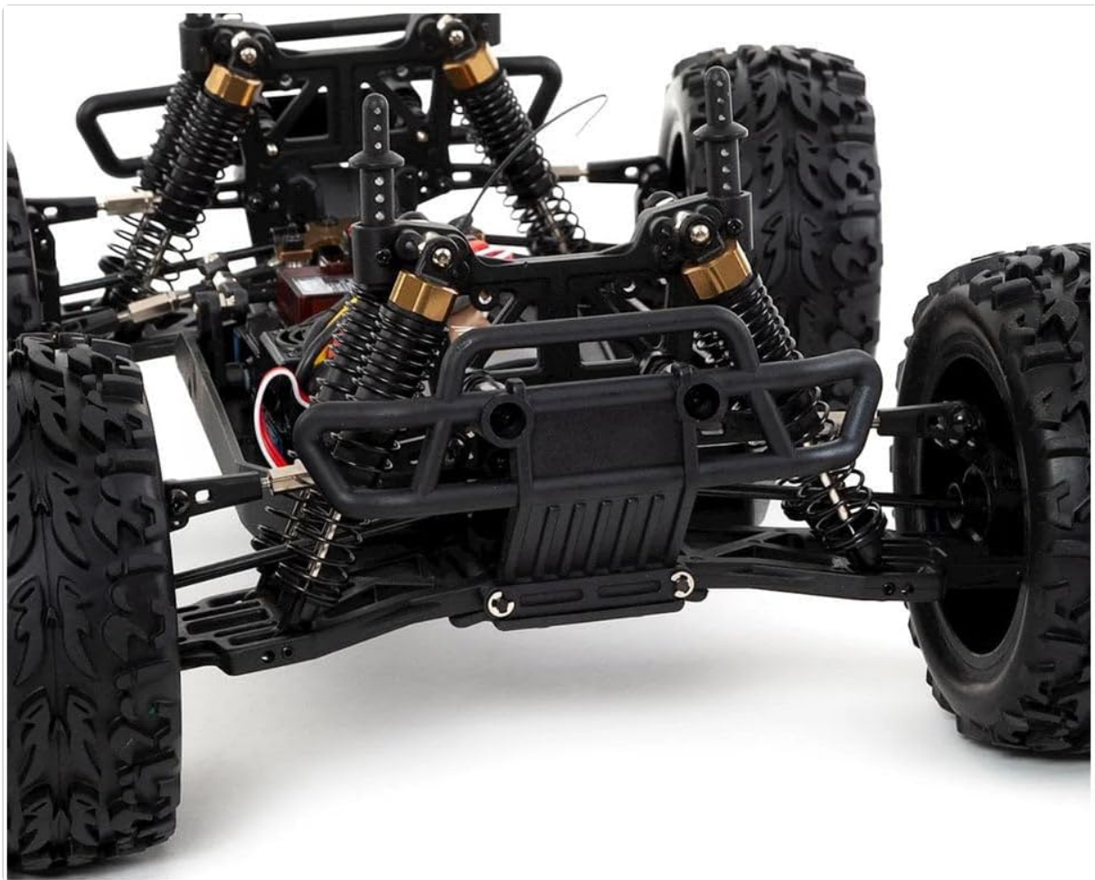
Figure 5: Close-up view of the front suspension and bumper assembly of the Maverick Strada MT. This image highlights the robust construction of the shock absorbers and the protective front bumper.
