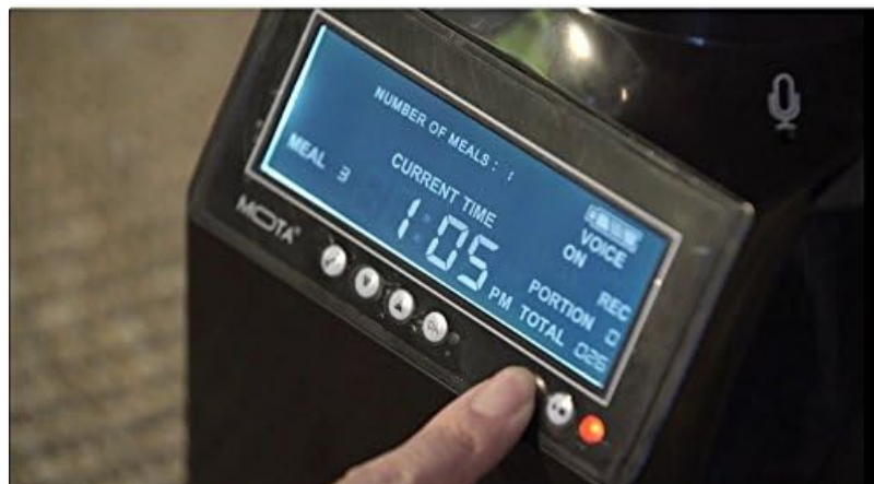
Figure 4: A detailed view of the dispenser's LCD screen and control buttons, illustrating the user interface for setting time and programming meals.
