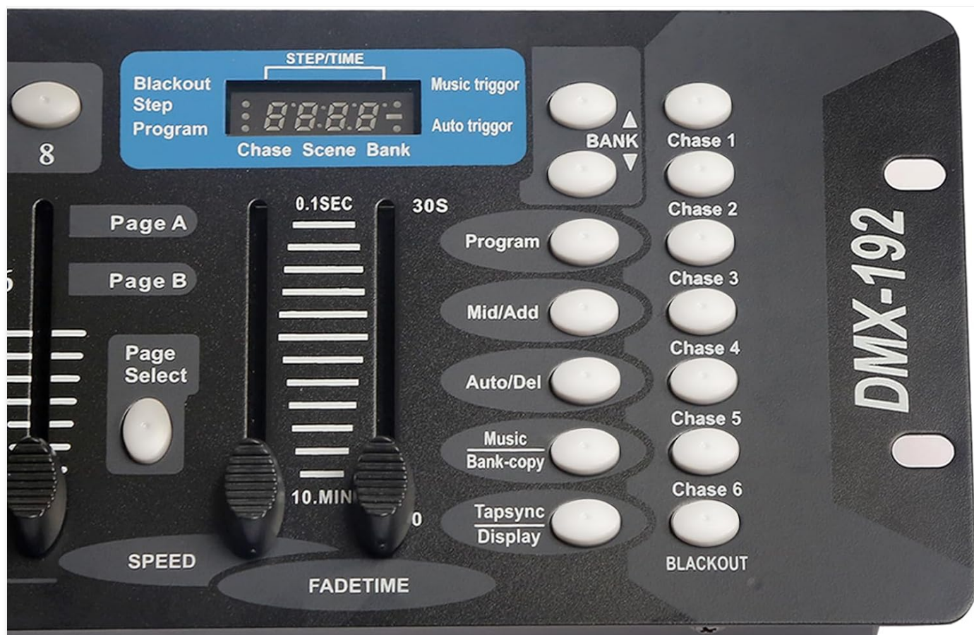
This detailed view focuses on the right side of the control panel, showing the Scene buttons (1-8), Chase buttons (1-6), Program button, MIDI/Add, Auto/Del, Music/Bank-copy, Tapsync/Display, and Blackout button. The digital display for step/time is also visible.
