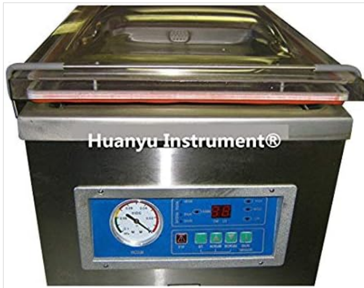
Image 1: Front view of the Huanyu DZ260 Automatic Vacuum Sealer, showing the main unit and the control panel with a pressure gauge and digital display.
