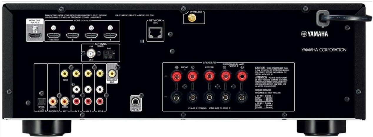
Image: The rear panel of the Yamaha RX-V481 receiver, displaying various ports including HDMI inputs/output, speaker terminals, audio inputs, and antenna connections.
