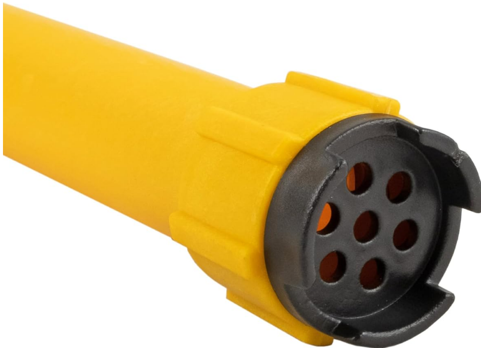
Figure 3: Close-up view of the bung adapter, designed to fit 15, 30, and 55 gallon drums with 1.25" and 2" NPT bung fittings.
