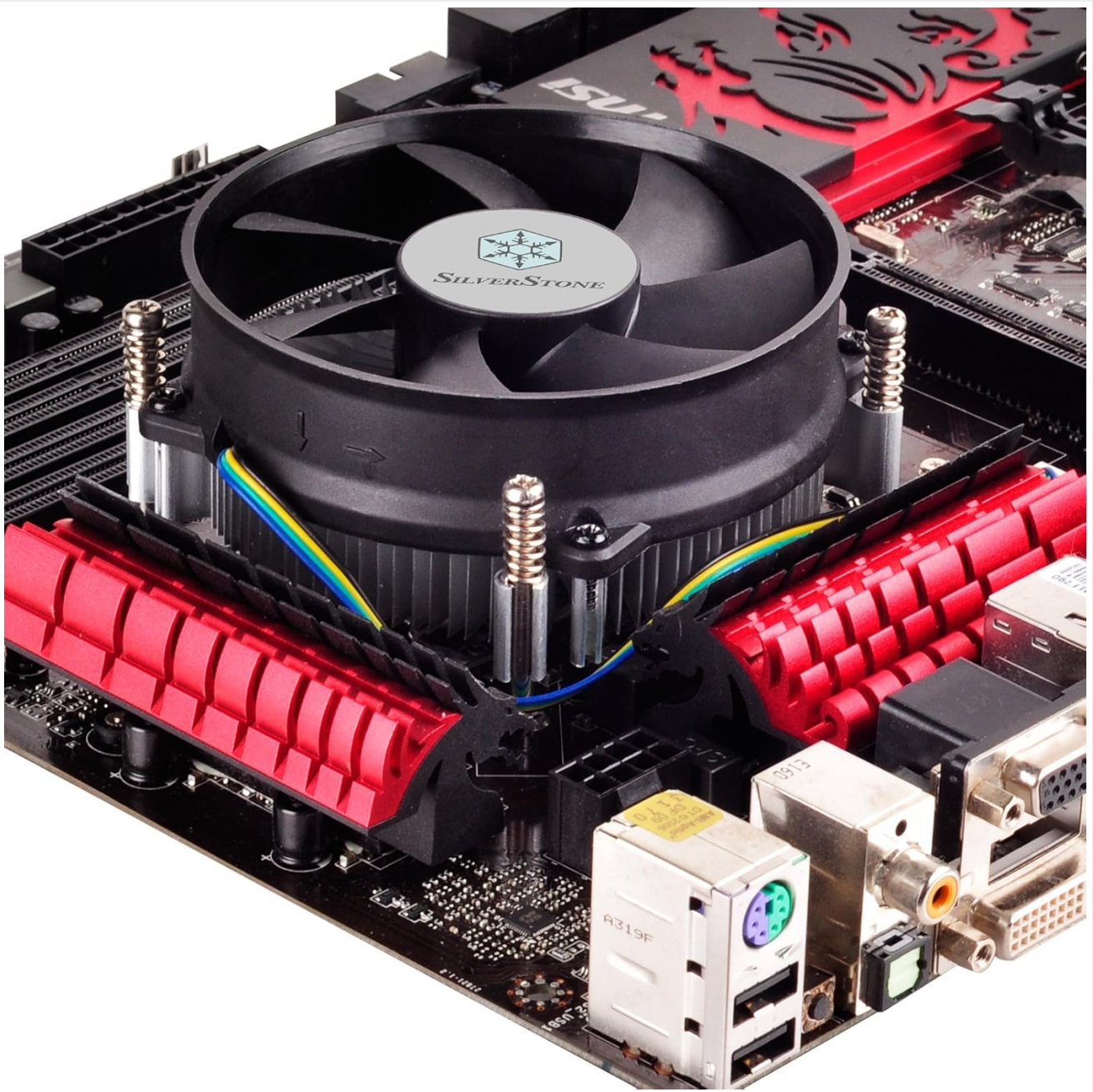
Figure 3: Top view of the CPU cooler correctly installed on a motherboard.
