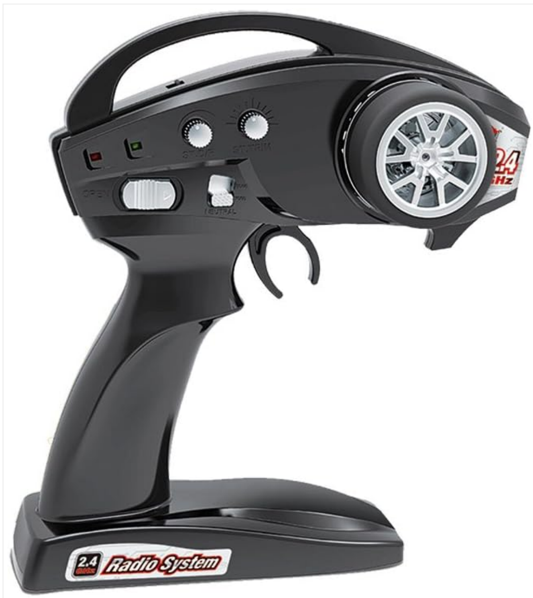
Image 4.1: The 2.4 GHz wireless remote control for the Dune Buggy.
