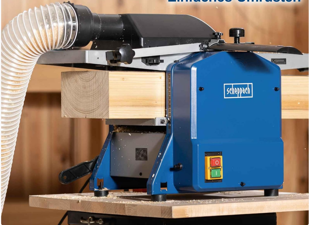
Figure 5: Thicknessing function in action
