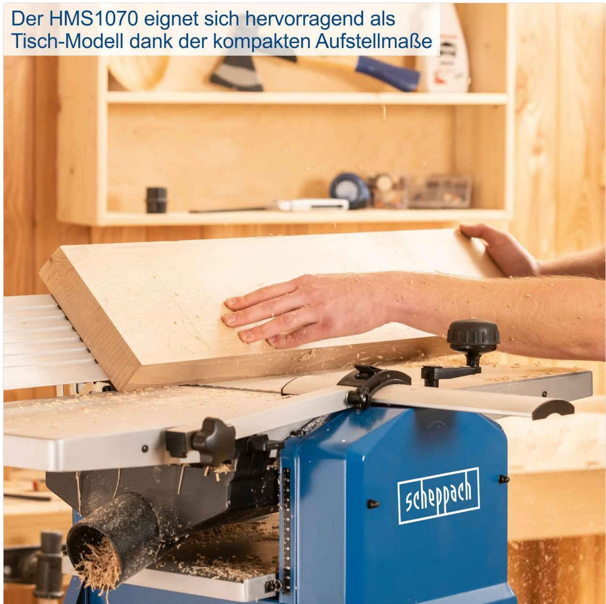
Figure 2: Demonstrates the planer in use, with a user feeding a wooden board for surface planing. This highlights the practical application and ergonomic design.
