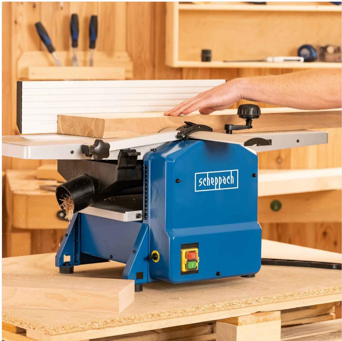
Figure 7: Another operational view, showing the planer actively processing wood and highlighting the dust extraction port for a cleaner workspace.
