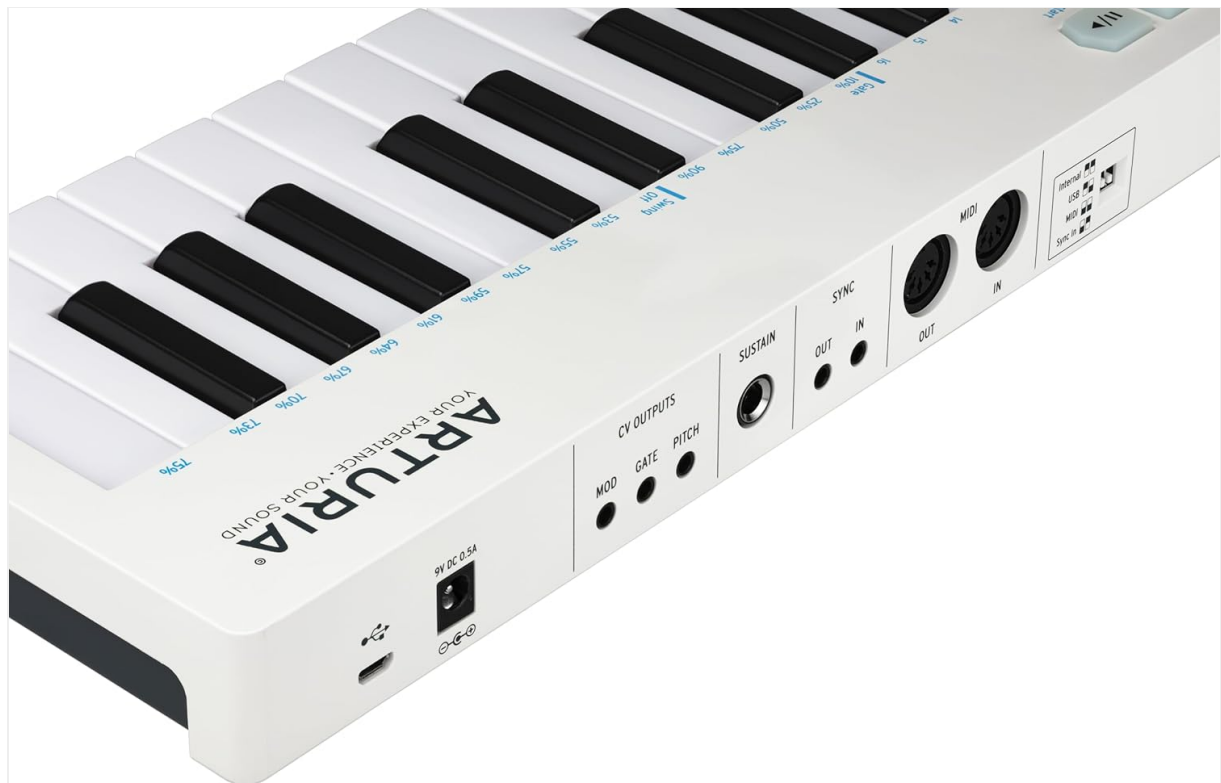
Figure 2: Rear panel connections including USB, Sustain, MIDI In/Out, Sync, and CV Outputs.
