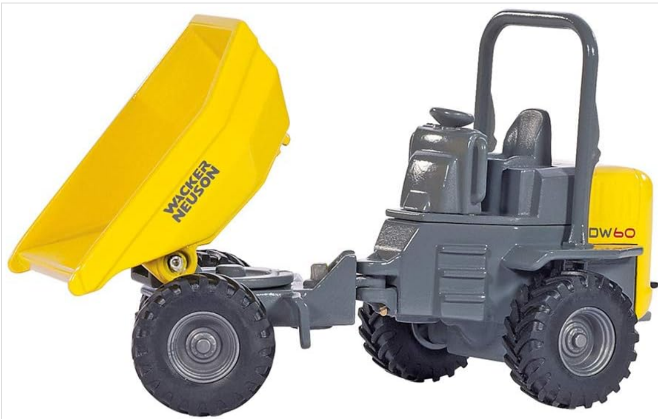
Figure 5.2: The dumper with its metal trough in the tipped position, ready for unloading.
