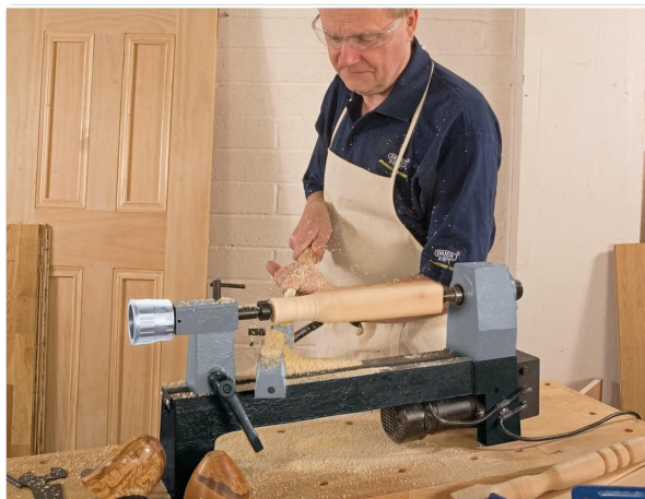
Image 2: A user demonstrating the operation of the wood lathe, shaping a workpiece.
