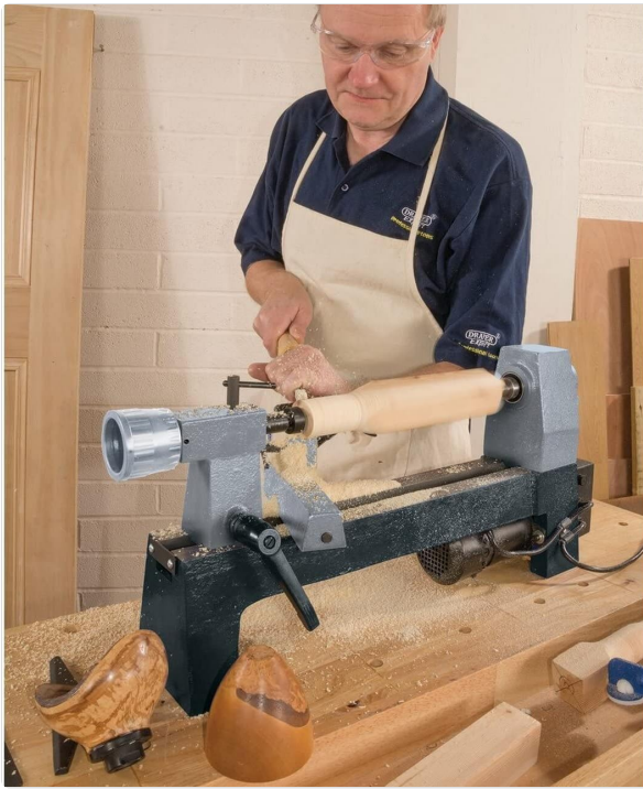
Image 3: Detailed view of the turning process, showing the tool rest and workpiece.
