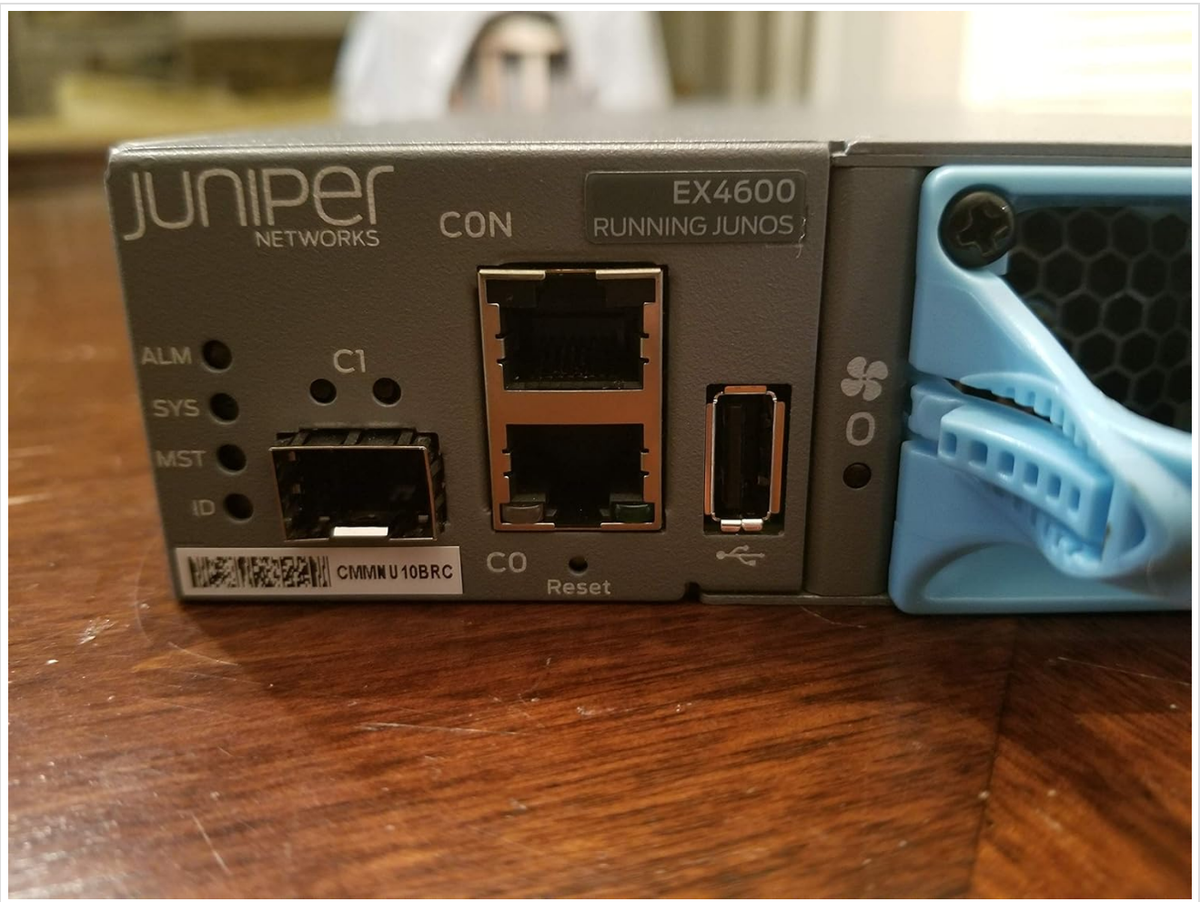
Image Description: A close-up view of the management section of the EX4600 switch. It shows the console port (CON), a management Ethernet port (C0), a USB port, and LED indicators for Alarm (ALM), System (SYS), Master (MST), and ID. The model number EX4600 is clearly visible.
