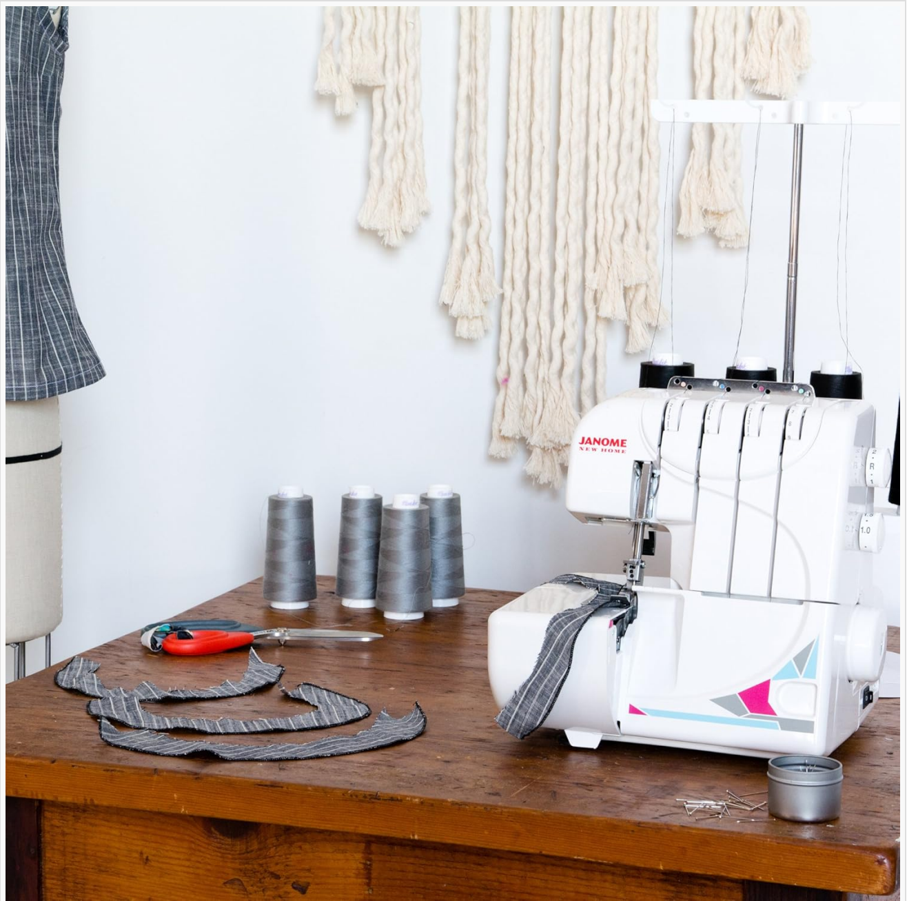
Figure 3: The serger positioned on a workspace, highlighting its overall size and the thread stand with multiple spools.
