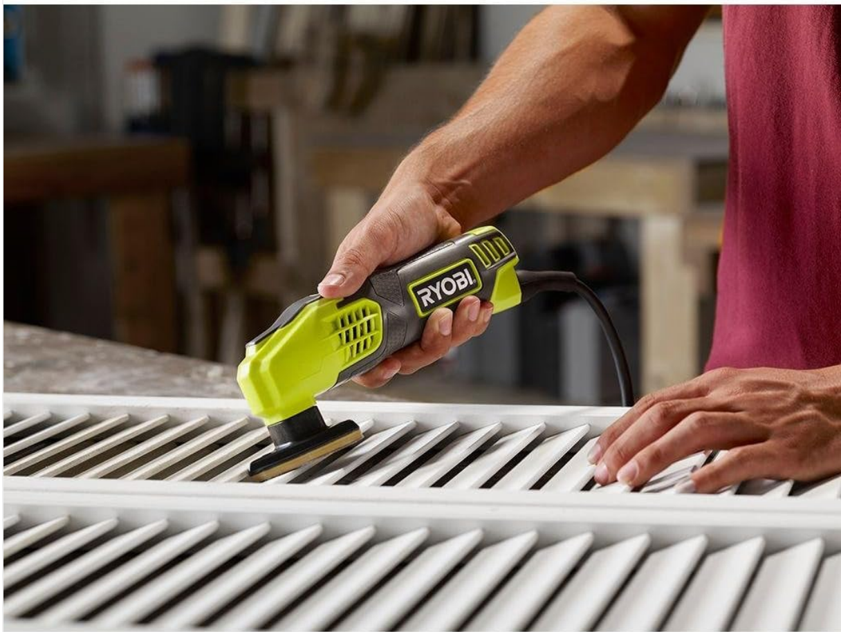
Figure 4: Demonstrating the use of the detail sander on intricate louvers, highlighting its ability to reach tight spaces.
