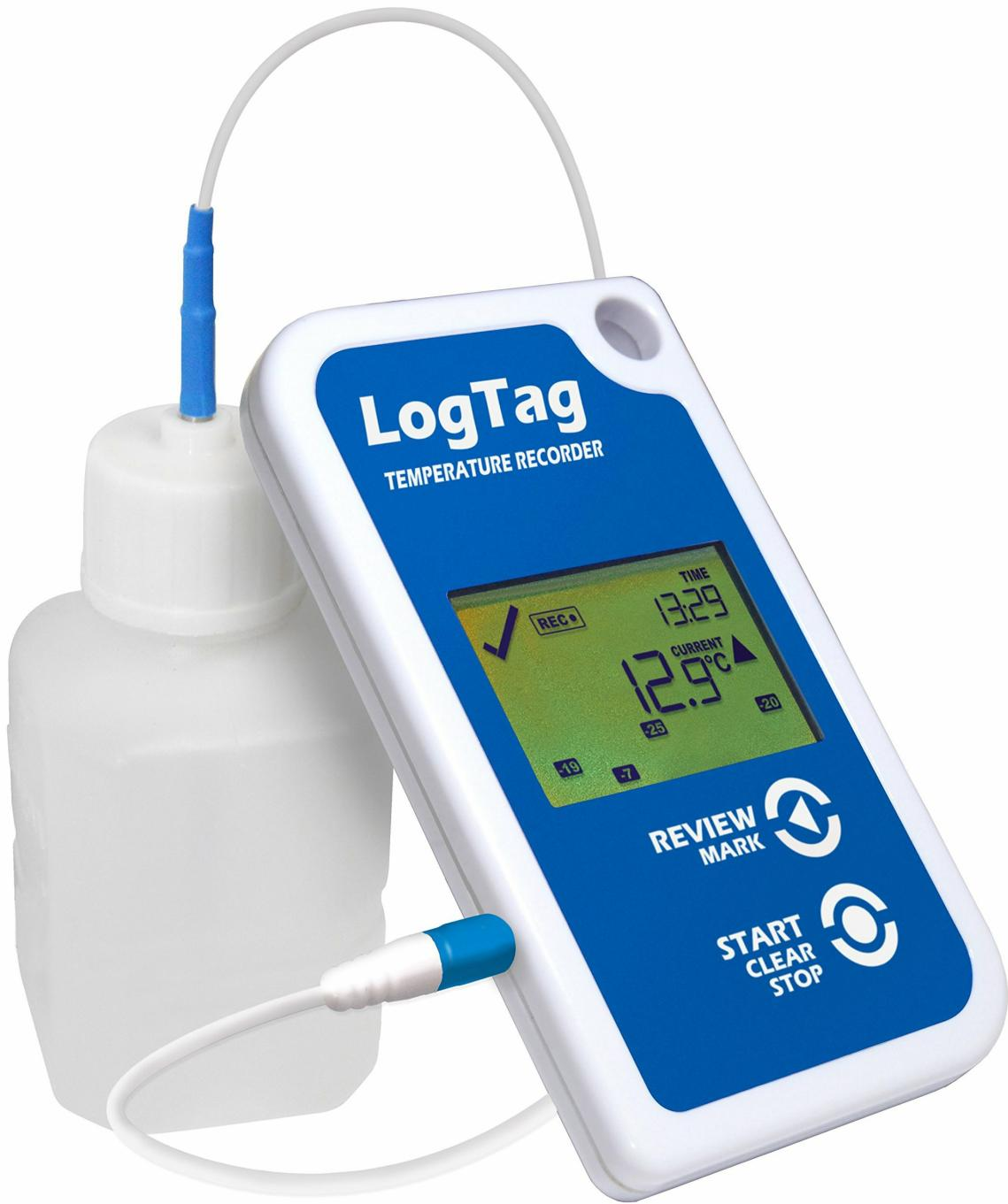
This image shows the LogTag TRED30-16R temperature data logger connected to an external probe, which is inserted into a glycol buffer bottle. The logger displays temperature readings and operational status.
