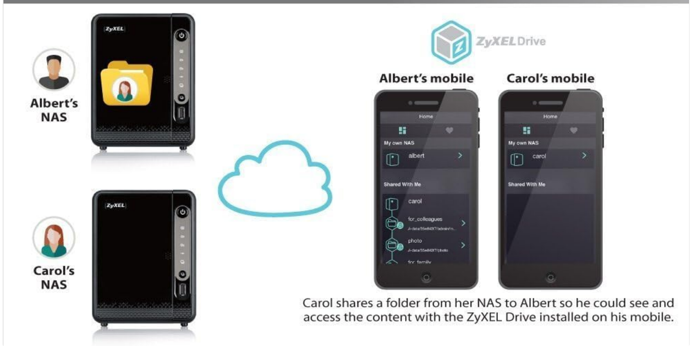
Figure 3.2: Diagram demonstrating how the ZyXEL Drive app facilitates easy remote access to your NAS from mobile devices, enabling sharing between users.
