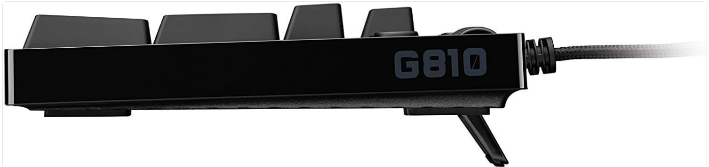
Figure 2: Side Profile of the G810 Keyboard. This image illustrates the keyboard's side profile, highlighting the adjustable feet that allow for ergonomic tilt customization.
