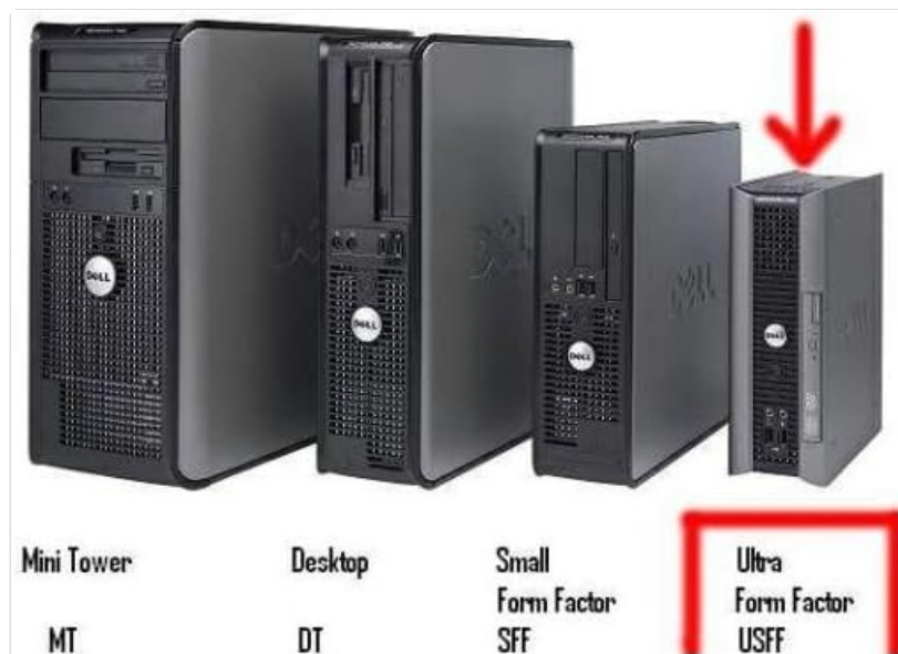
Figure 7.1: Various Dell Optiplex form factors. The Optiplex 760 is commonly available in Desktop or Small Form Factor (SFF) configurations.
