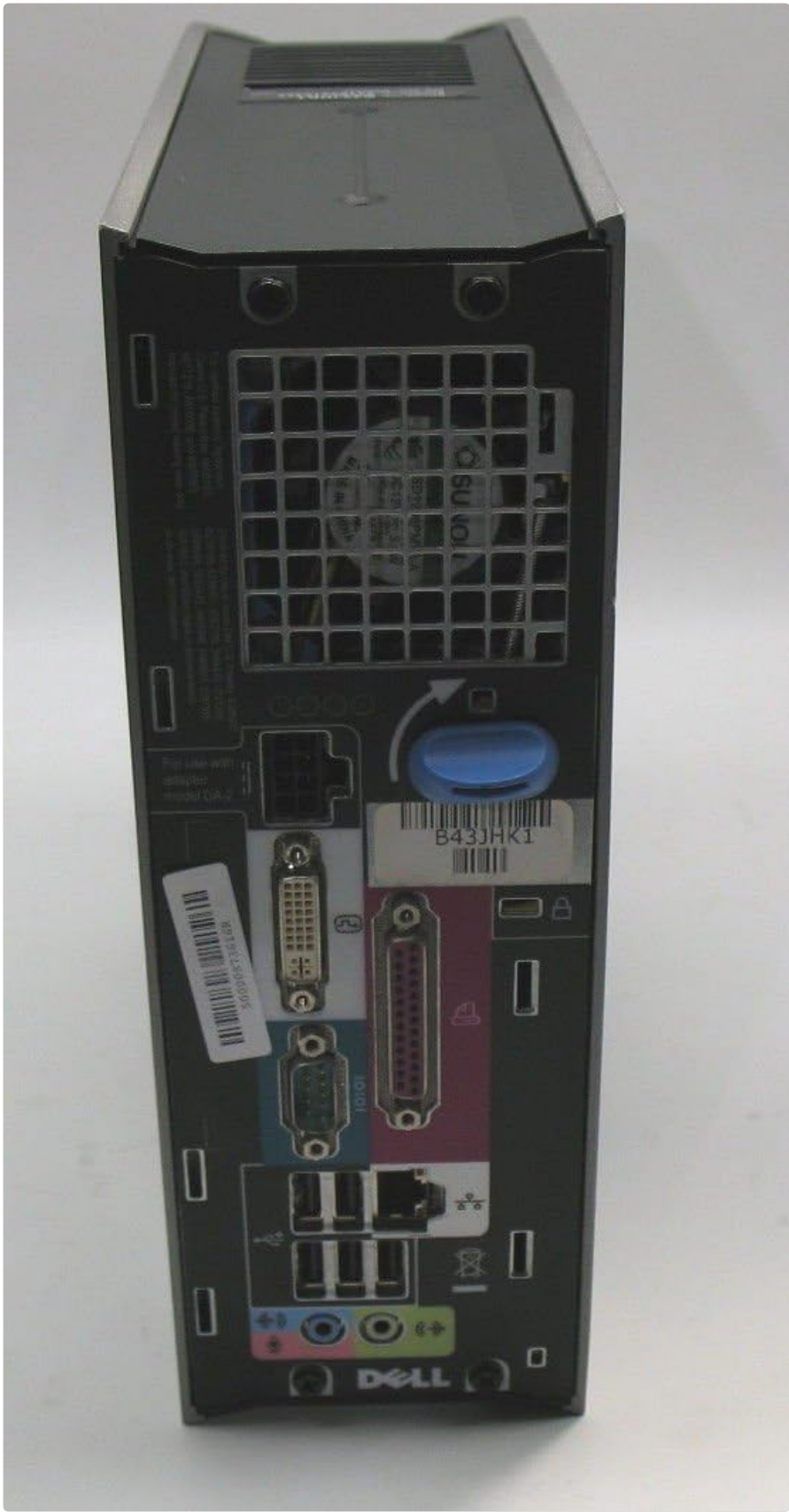
Figure 3.1: Rear ports of the Dell Optiplex 760, including USB, VGA/DVI, Ethernet, and audio ports.
