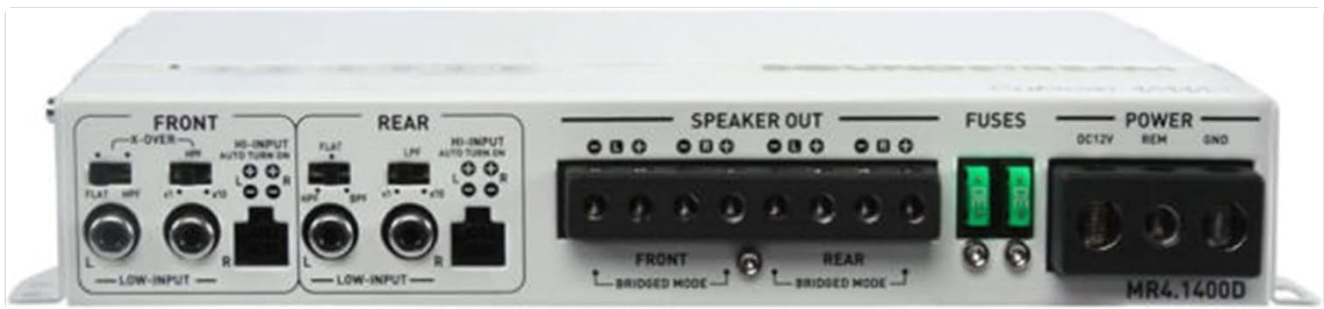
Figure 4.1: Rear panel view of the Soundstream MR4.1400D amplifier, showing all input and output terminals, fuses, and control knobs. From left to right, it displays Front and Rear input sections (Low-Input RCA, Hi-Input), Speaker Output terminals, Fuses, and Power terminals (DC12V, REM, GND).
