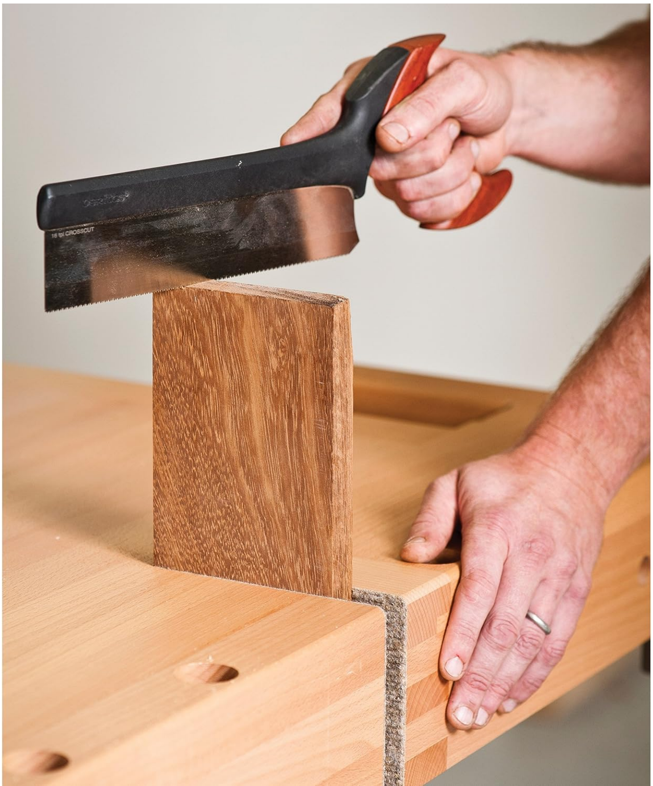
Figure 3: Demonstrates using the workbench to secure a piece of wood for sawing, highlighting the stability provided by the clamping mechanism.
