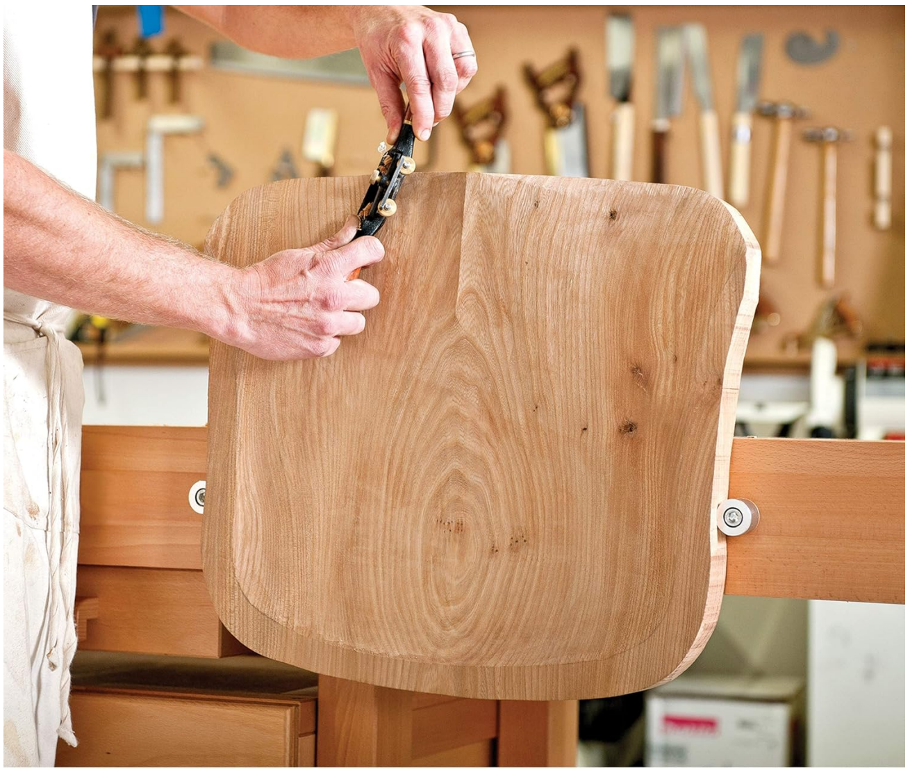
Figure 5: Shows a curved wooden piece being worked on with a spokeshave, demonstrating the versatility of the workbench's clamping for irregular shapes.
