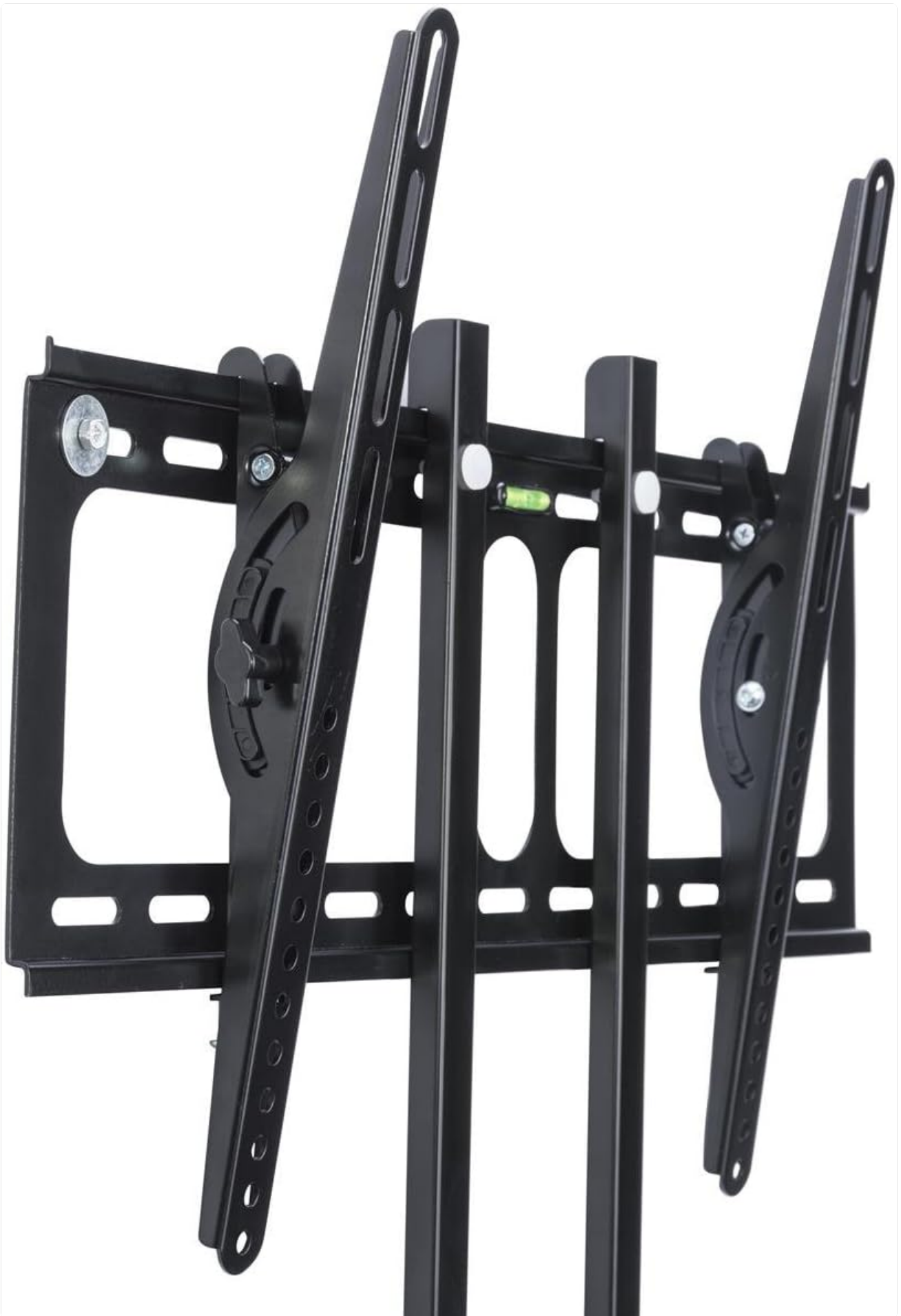
Image: A side view of the TV mount, highlighting the adjustable tilt mechanism on the TV brackets, which allows for angle adjustments after mounting.
