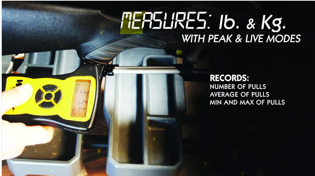
Image 3.2: The gauge's display indicating measurement units (lb. & Kg.) and recording capabilities for peak, live, average, min, and max pulls.
