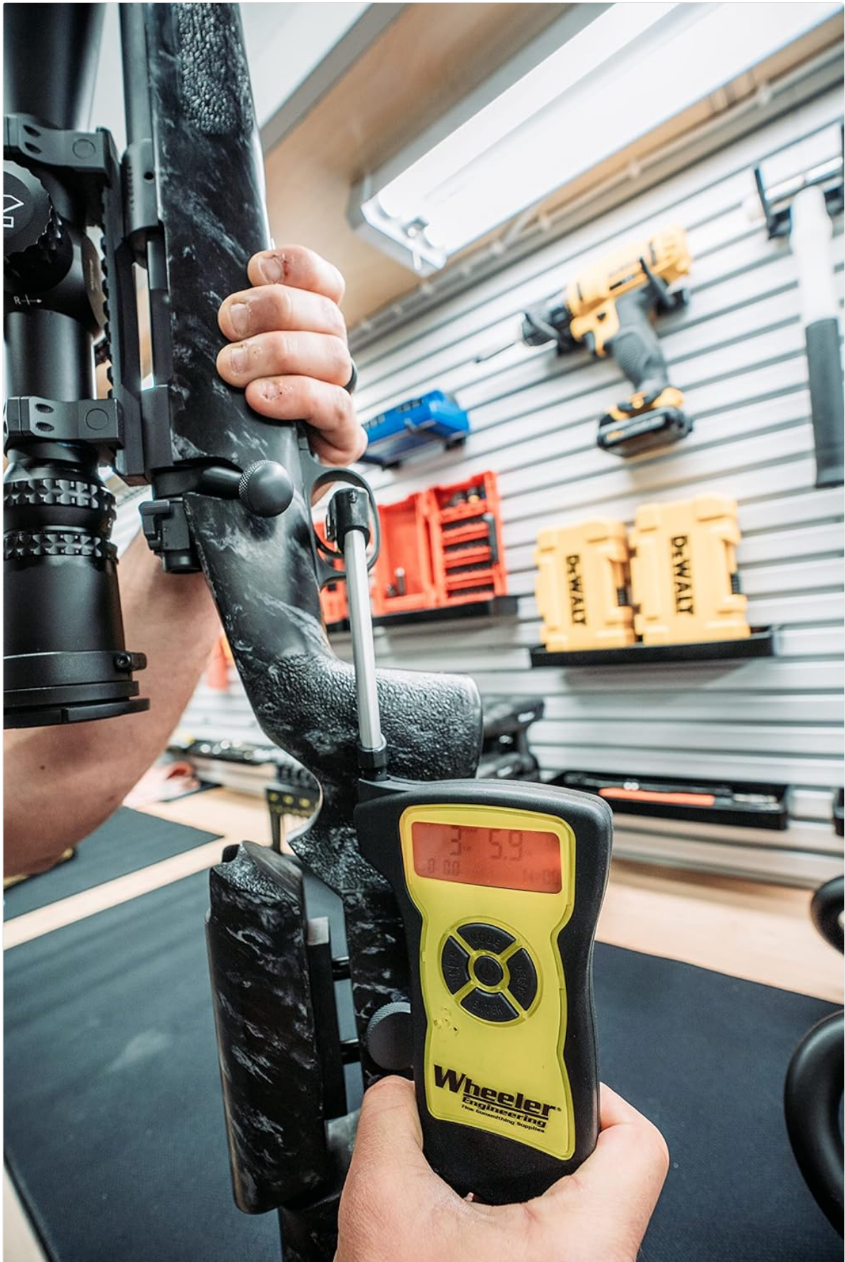
Image 3.1: Demonstrating the Wheeler Digital Trigger Pull Gauge measuring the trigger pull of a rifle.
