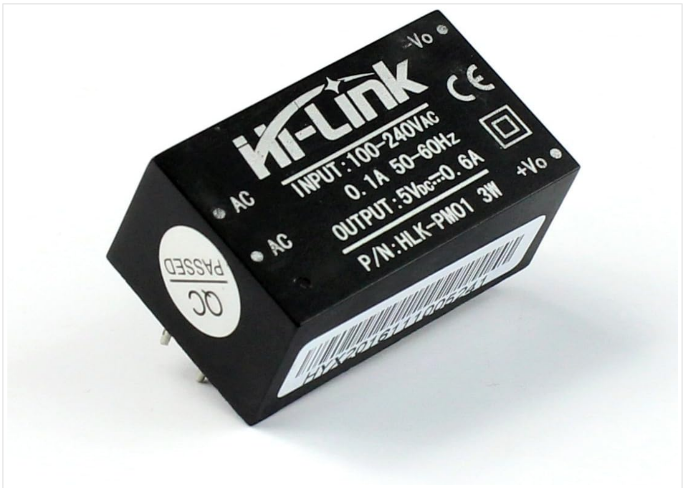
Figure 2: Angled view of the HLK-PM01 module, highlighting the input (AC) and output (+Vo, -Vo) pins.
