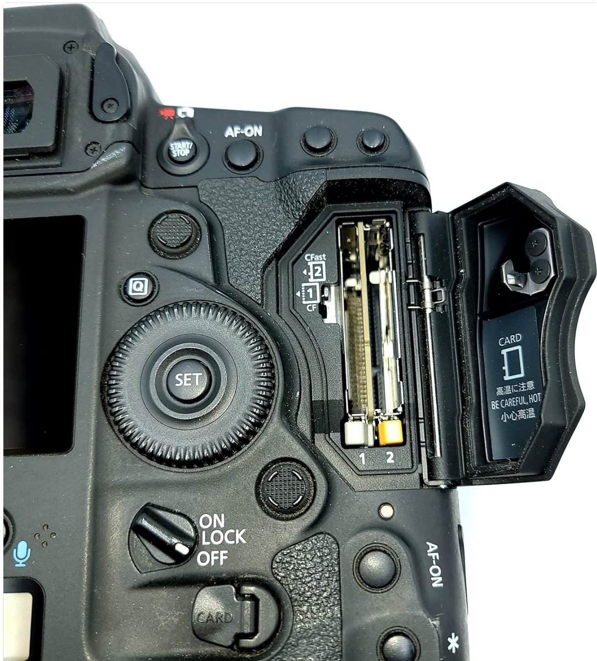
Figure 3.2: Detailed view of the dual memory card slots, indicating CFast 2.0 and CF compatibility.
