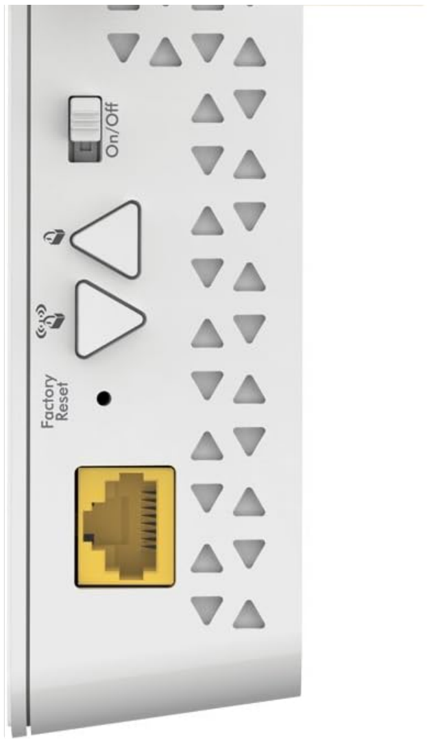
Figure 4: Side view of the PLW1000, highlighting the Ethernet port, Factory Reset button, and On/Off switch for WiFi.
