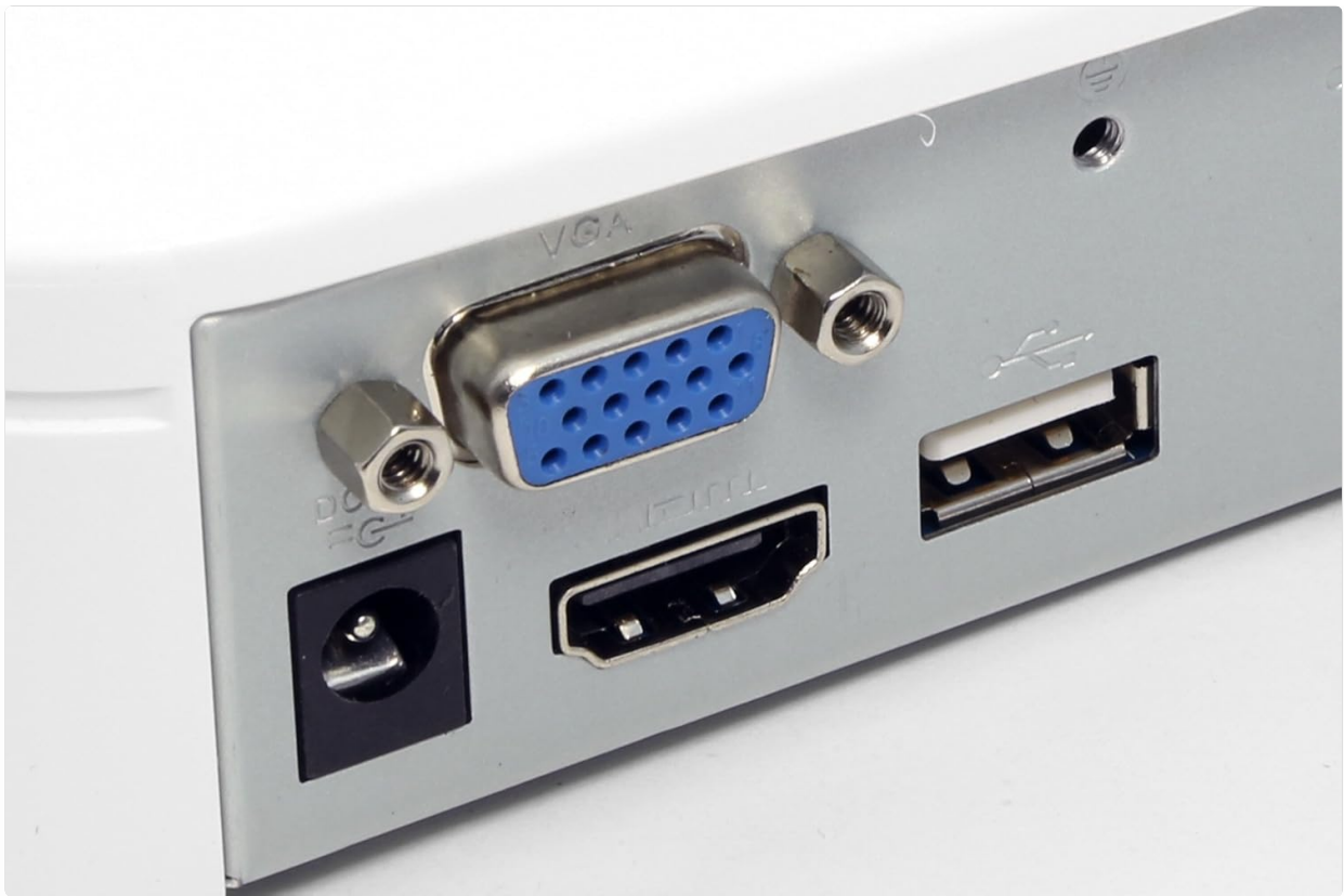
Image 3.1.2: Receiver rear panel with DC power, VGA, HDMI, and USB ports.
