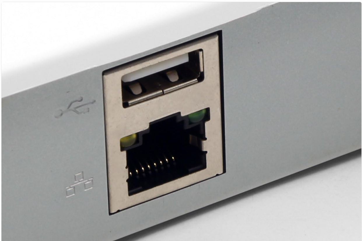
Image 3.1.3: Receiver rear panel with Ethernet and USB ports.
