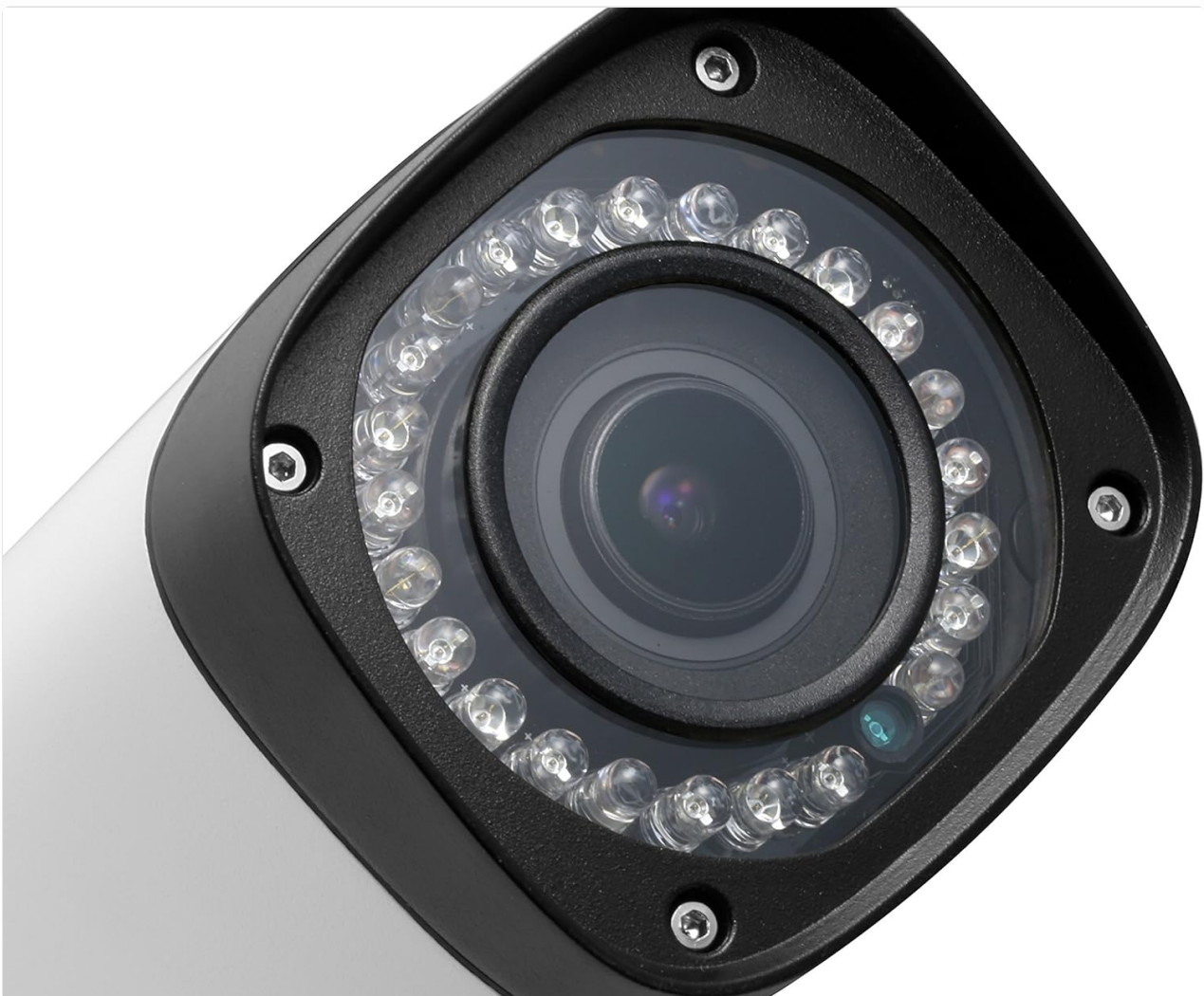
Image 3.2.2: Detailed view of the bullet camera lens, highlighting the infrared LEDs for night vision.
