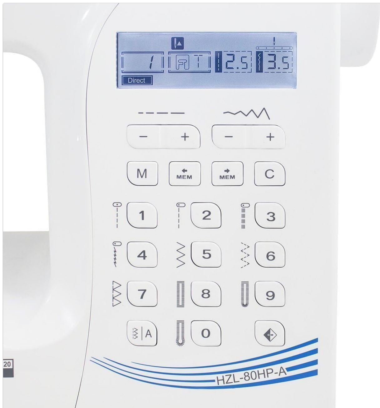
Figure 3.2: Close-up of the control panel with LCD screen and stitch selection buttons.
