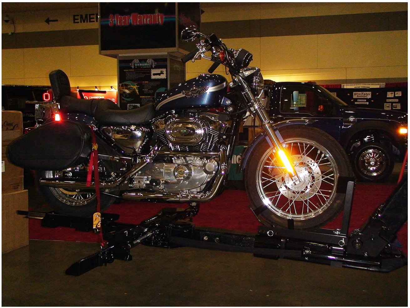
Figure 4: A motorcycle positioned and secured on the CONDOR Self-Loader, demonstrating the upright stability provided by the wheel chock.
