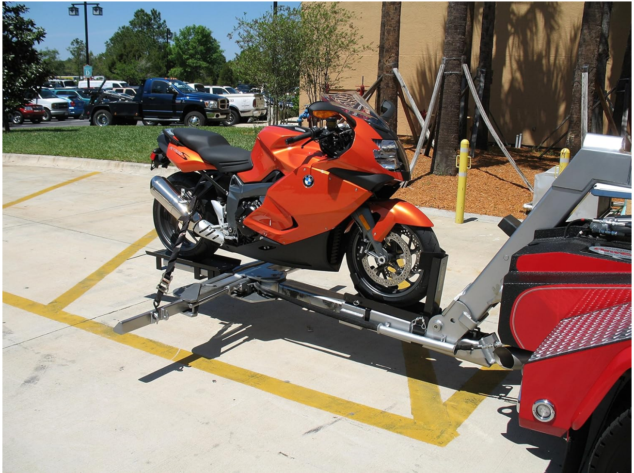
Figure 7: A motorcycle fully secured on the CONDOR Self-Loader, demonstrating its readiness for transport by a wrecker.
