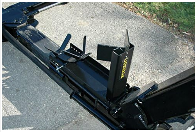
Figure 3: The CONDOR Self-Loader fully installed and extended from the rear of a wrecker, ready for motorcycle loading.
