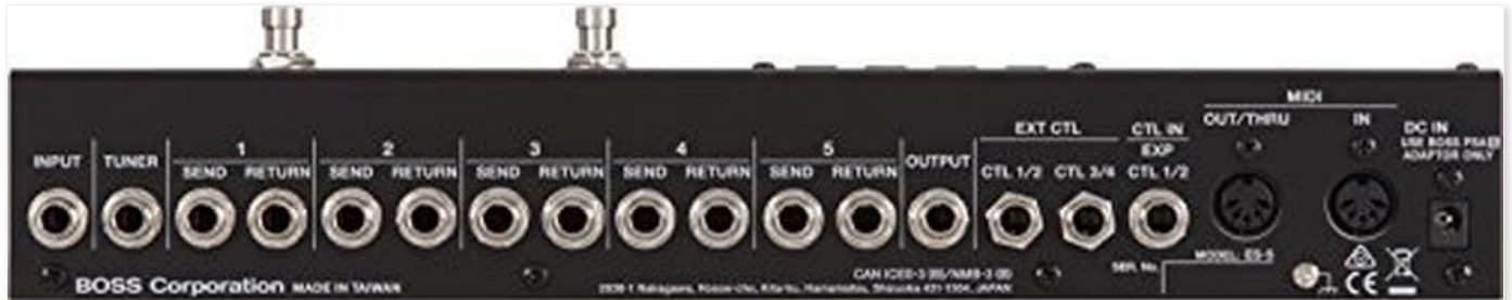
Figure 2: Rear panel of the BOSS ES-5, showing INPUT, TUNER, SEND/RETURN loops (1-5), OUTPUT, EXT CTL, CTL IN/EXP, MIDI (OUT/THRU), and DC IN jacks.
