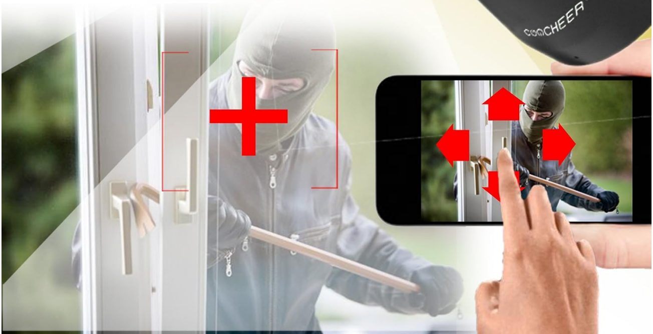
Figure 5.1: Illustration of the motion detection feature, showing how the camera detects movement and can trigger an alarm or recording.
