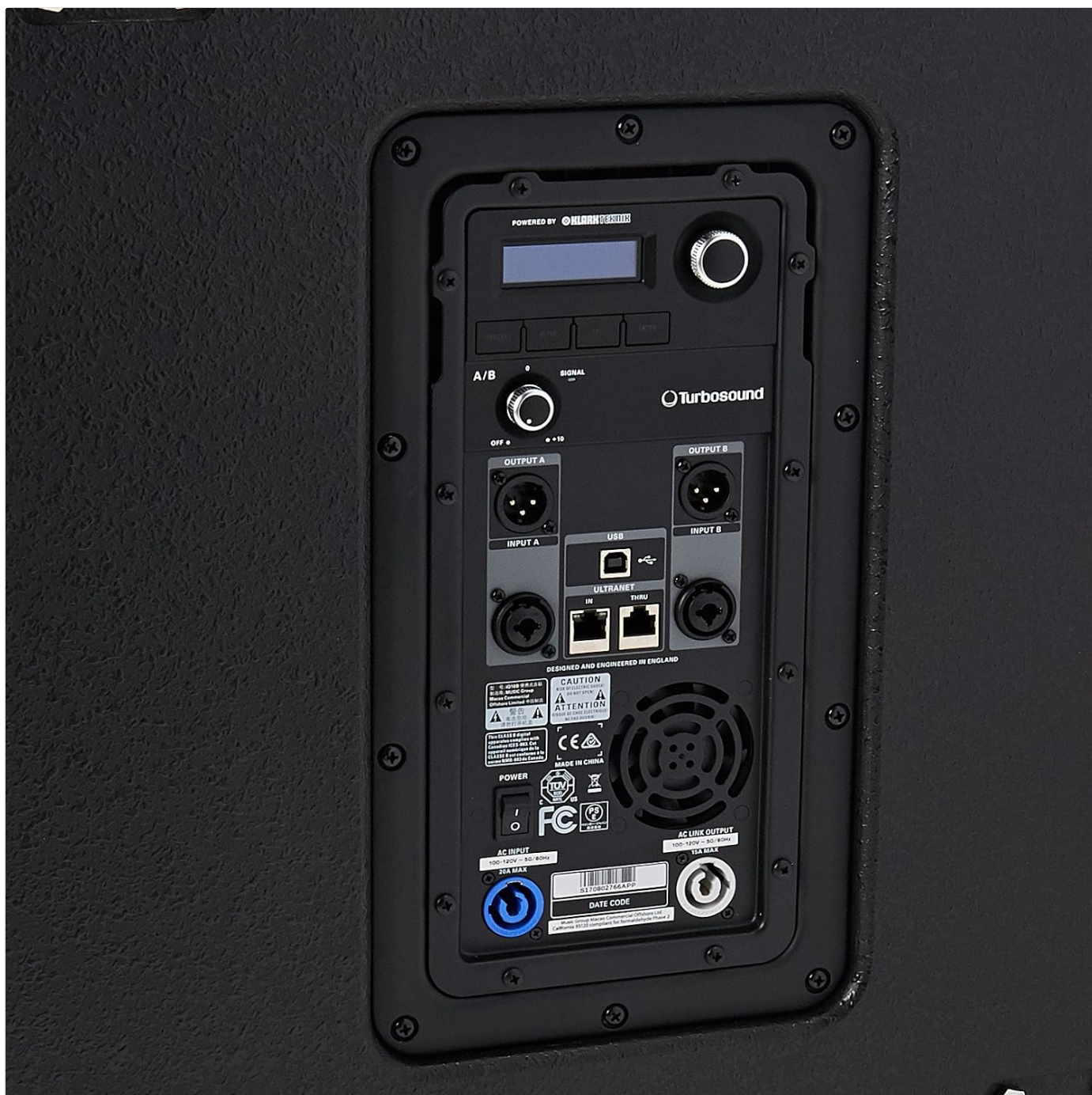
Figure 2: Rear panel showing input/output connections and controls.
