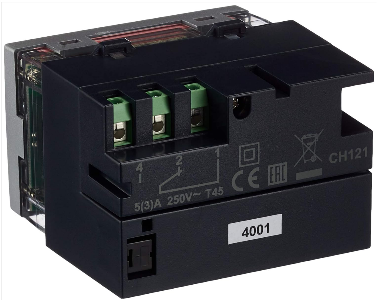
Image 4.1: Rear view of the Fantini Cosmi CH121 thermostat, showing the wiring terminals (labeled 1, 2, 4) and specifications such as 5(3)A 250V~ T45, indicating its electrical rating and temperature class.
