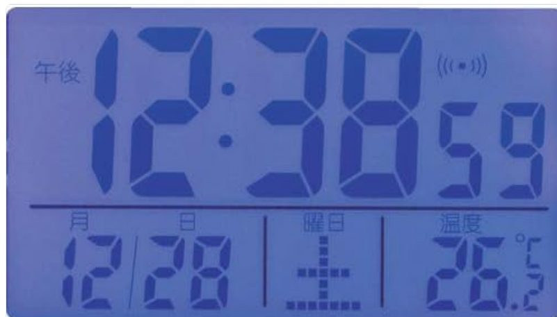
Figure 4.2: Close-up of the ADESSO SN-01 Alarm Clock's digital display, showing the time (12:38), seconds (59), radio wave reception indicator, date (12/28), day of the week, and temperature (26.7°C).
